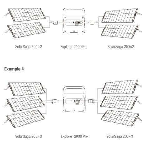
Note: When charging with more than three solar panels, two connectors are required. Make sure both connectors connect the same amount of solar panels to avoid damaging or failing to charge the power station.
