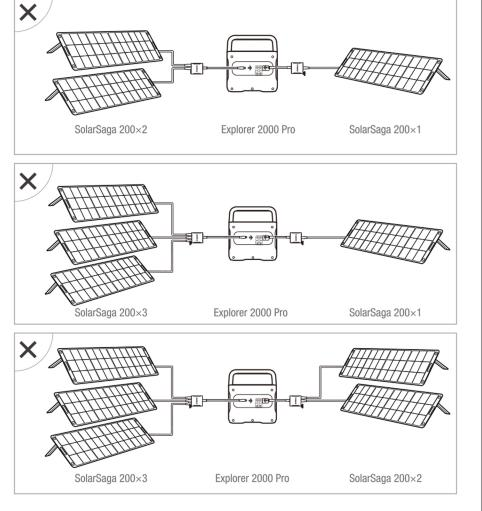
Caution: When the two inputs are used at the same time, please make sure to use the same type of solar panel and the number of solar panels in the two inputs must be the same to avoid damage or charging problems of the equipment due to inconsistent voltages of the two channels.
